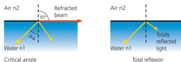
There comes a time when all of the rays are reflected, this happens when the angle of incidence is equal to or greater than the critical angle  $\alpha_{crit}$ , which is defined by the ratio of the two indices of refraction:
