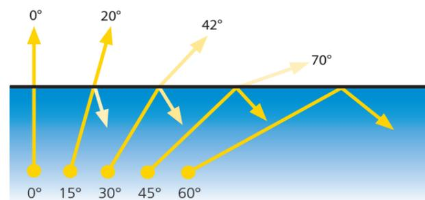
A more detailed picture below shows the case where light impinges under such special angle that the refracted beam makes an angle of 90° with the surface normal.
